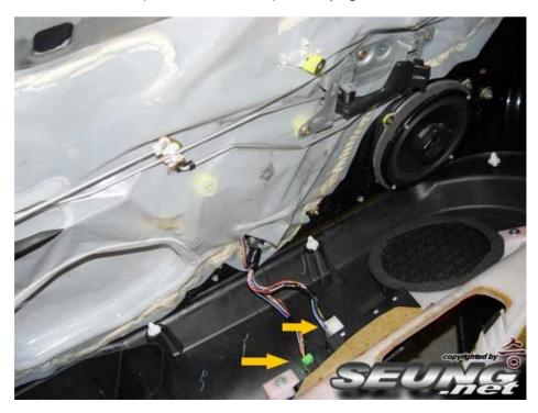
gently pull the door panel off, and remove two wire sockets, one for window control, and the other for mirror controls. (pass. side door panel has only one socket.)
