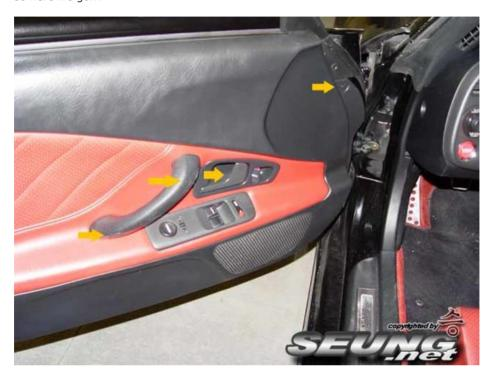
first remove the door panels... arrows indicate the tap/ bolts you have to remove. one behind door latch, two on door handles, and a tap right below the front of the window.
